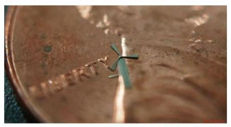
Developed by Smitha Rao and J.C. Chiao, the windmills blend origami concepts into conventional wafer-scale semiconductor device layouts so complex 3D movable mechanical structures can be self-assembled from 2D metal pieces utilizing planar multilayer electroplating techniques that have been optimized by WinMEMS Technologies Co.
