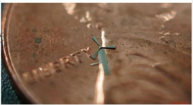
semiconductor device layouts so complex 3D movable mechanical structures can be self-assembled from 2D metal pieces utilizing planar multilayer electroplating techniques that have been optimized by WinMEMS Technologies Co.
