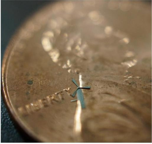
Two UT Arlington engineers have invented a tiny, working windmills. They propose creating a field of these windmills on a cell phone sleeve, and using them to recharge cell phone batteries.
