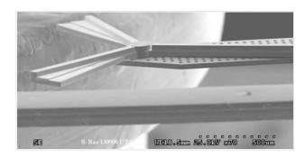
These micro-windmills – called horizontal axis wind turbines – have a three-bladed rotor that is 1.8 mm in diameter, 100 microns thick, and are mounted on a tower about 2 mm tall mount. Despite their tiny size, the micro-windmills can endure strong winds, owing to being constructed of a tough nickel alloy
