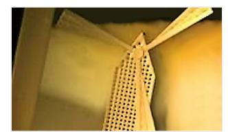
The windmills were crafted using origami techniques that allow two-dimensional shapes to be electroplated on a flat plane, then self-assembled into 3D moving mechanical structures. Rao and Chiao created the windmill for a Taiwanese superconductor company called WinMEMS, which developed the fabrication technique. And as Rao stats, they were interested in her work in micro-robotics:
