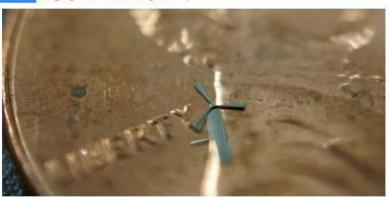
Above is a micro-windmill that University of Texas Arlington researchers suggest could someday be used to charge mobile electronics if they were embedded en masse on the device's case. The MEMS (micro-electromechanical systems) are fabricated using recesses similar to the way integrated circuits are manufactured combined with origami-like self-assembly techniques.
