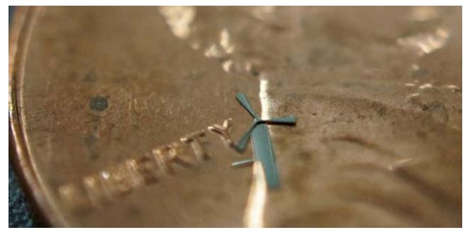
Above is a micro-windmill that University of Texas Arlington researchers suggest could someday be used to charge mobile electronics if they were embedded en masse on the device's case. The MEMS (micro-electromechanical systems) are fabricated using recesses similar to the way integrated circuits are manufactured combined with origami-like self-assembly techniques.
