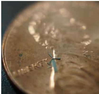
An actual micro-windmill sits atop a penny. (Credit: University of Texas at Arlington)
