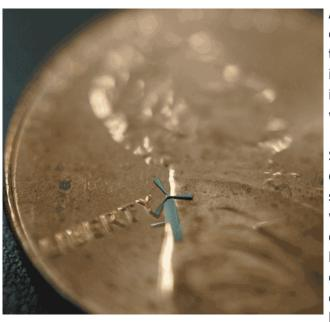
A UT Arlington research associate and electrical engineering professor have designed a micro-windmill that generates wind energy and may become an innovative solution to cell phone batteries constantly in need of recharging and home energy generation where large windmills are not preferred.
