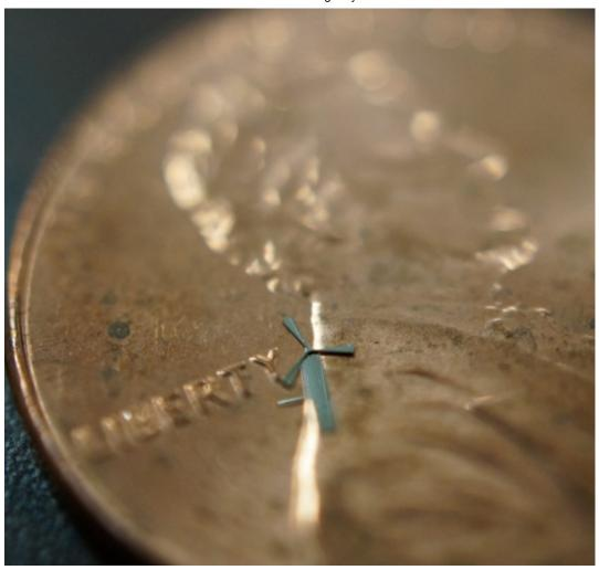
The new micro windmills measure about 1.8 mm at their widest point, that miniature sizing means that roughly ten or so of them can be fitted onto something the size of a single grain of rice — thereby potentially providing a notable fraction of the energy used by portable electronics. The windmills are turned simply by the force of the air as the device that they are installed on is moved around during everyday usage.
