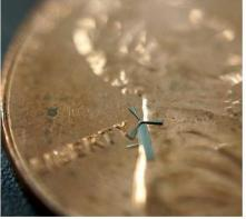
However, these new devices. microwindmills, do not tower over large plots of land. Instead, they measure only 1.8 millimeters wide. According to J.C. Chiao, cocreator and electrical engineering professor at the University of Texas at Arlington, the microwindmills are so tiny that 2,040 of them could fit on an iPhone 4.
