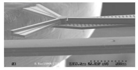
The miniature turbines measure at 1/15 of an inch at its widest, and will generate a small electrical charge from ambient wind. The structures "blend origami concepts into conventional wafer-scale semiconductor device layouts so complex 3-D movable mechanical structures can be self-assembled from two-dimensional metal pieces, utilizing planar multilayer electroplating techniques."
