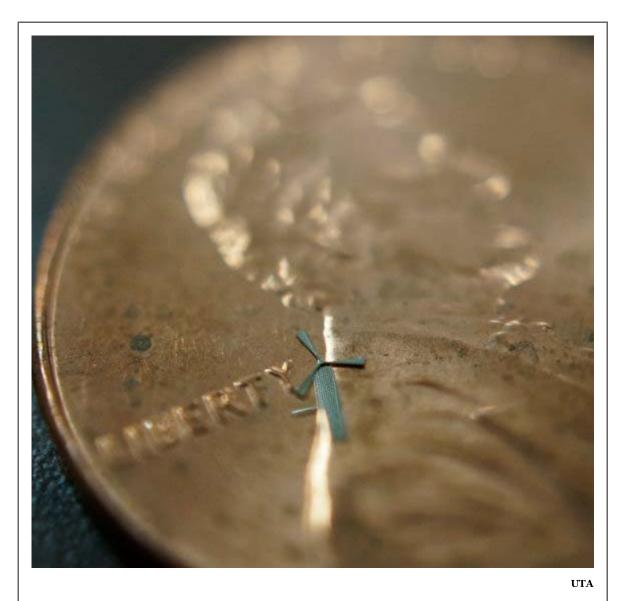
Think of it as the intersection between origami and semiconductor manufacturing. Researchers at the University of Texas at Arlington have invented a nickel-alloy windmill so tinv that 10 of them could be comfortably anchored to a grain of rice.
