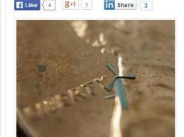
Researchers at University of Texas Arlington (UTA) have developed a new minute 'micro-windmill' that generates wind energy, which could be used to charge cell phone batteries.
