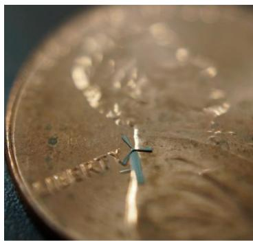
Flat panels with thousand of windmills could be made and mounted on the walls of houses or building to harvest energy for lighting, security or environmental sensing and wireless communication
