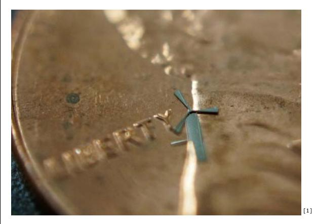
Researchers at the <u>University of Texas at Arlington</u> [2] are working on the world's tiniest <u>wind farm</u> [3] that could fit on a grain of rice and <u>charge your smartphone</u> [4]! The teeny tiny windmill is just 1.88mm wide, and uses a miniscule electroplating system to generate spinning power. Headed by Smitha Rao and J.C. Chiao, the research team has partnered with <u>WinMEMS Technologies Co.</u> [5] to realize the baby windmill project.
