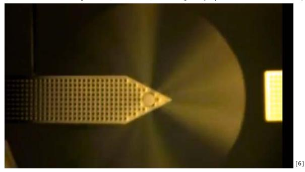
The super conducting tiny windmills [7] are made from resistant nickel alloy picked for its rigidity and durability. Each of the little mills is made using a technique similar to origami. The mini fan is self-assembled with wafer-scale semiconductor electroplating principles shrunk down to a bug's eye view. The 1.88mm fans are so small that ten of them could be placed on a grain of rice, working together as a miniature powerhouse.
