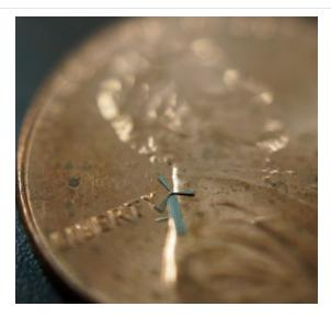
Researchers at UT-Arlington designed the micro windmill that is so small 10 of them could fit on a single grain of rice.
