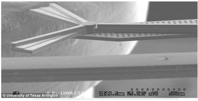
Each windmill, close up pictured, is made of flexible nickel alloy components capable of taking strong winds without breaking. They are so small that ten of them can fit onto a single grain of rice. Taiwanese fabrication foundry WinMEMS Technologies owns exclusive rights to sell the concept
