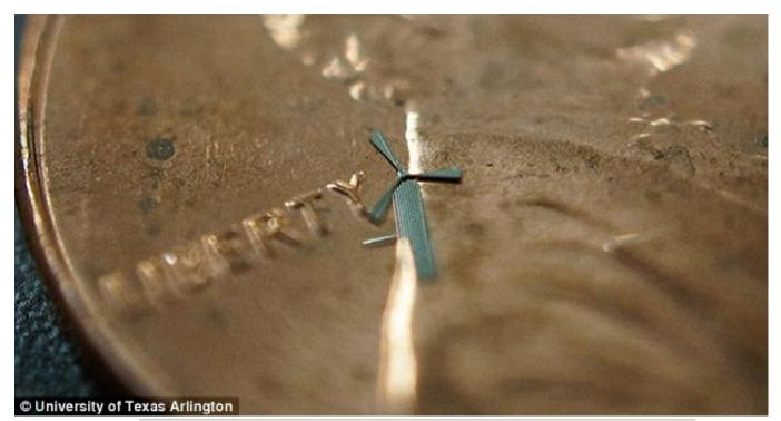
Researchers from Texas have developed a miniscule 'micro-windmill' that is just 1.8mm wide, pictured here on a U.S. penny, and can transform wind energy into electricity. The team claim hundreds of the nickel devices could be fitted to a phone case, and users could charge their phone simply by waving it in the air
