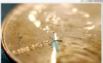
One of the micro-windmills is placed on a penny. Researchers in Texas envision embedding hundreds of them in a smartphone sleeve to provide a charge with the wind. Photo credit: University of Texas at Arlington
