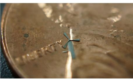
Researchers at the University of Texas at Arlington have come up with a way to build a nickel alloy windmill so small, 10 of them could be mounted on a grain of rice. And if all goes as planned, hundreds of the little things could end up in a case that charges up your smartphone.
