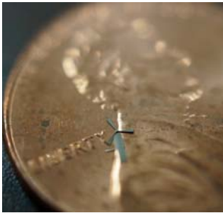
( http://thefutureofthings.com/wp-content/uploads/2014/01/microwindmill-penny_web.jpg ) Size of Micro-Windmill is smaller than a penny (Credit: UTA.edu)
