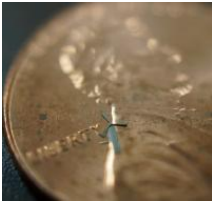
IMAGE: A micro-windmill is pictured on the face of a penny.
