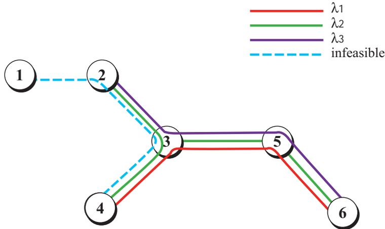
Figure 1: Unroutable 1-4 traffic due to wavelength-continuity constraints
